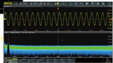
Real-time Spectrum Analysis Function 10,000 Hardware Accelerated FFTs/s
